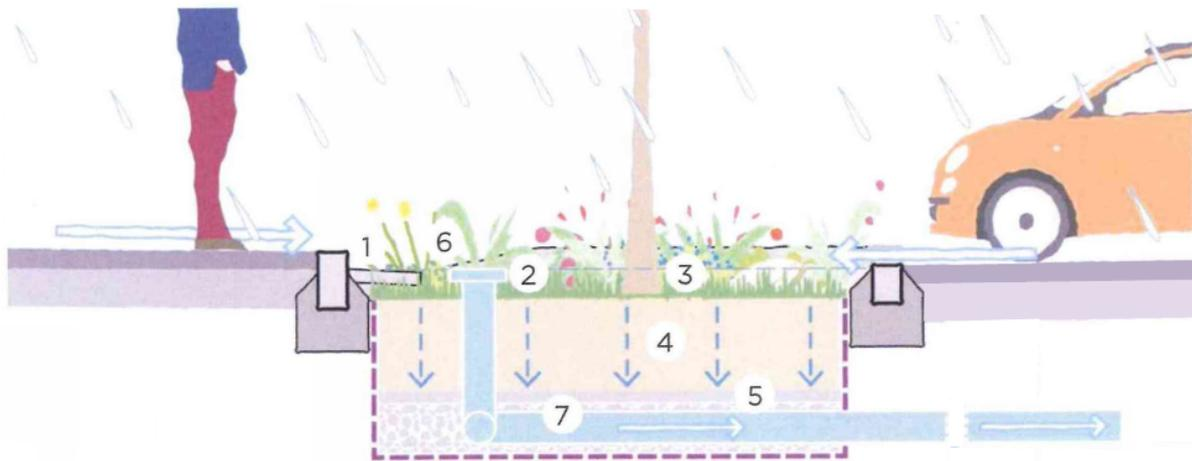
**Figure 4** Bioretention Tree Pit Raingarden
