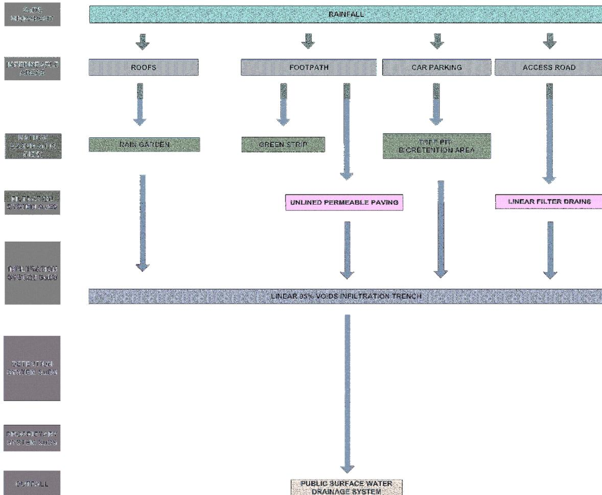
Figure 3 Proposed surface water treatment train
